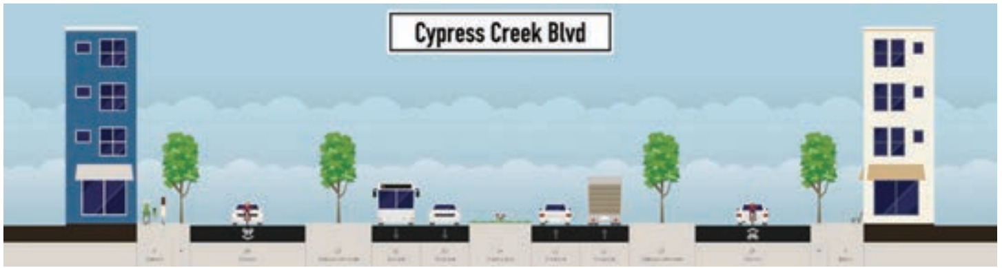
Figure 48: The Cypress Creek multiway boulevard (top image above) will be suitable for both people and vehicles. The multiway boulevard (top image below) is described in the National Association of City Transportation Officials Urban Street Design Guide. The bottom image below shows a typical multiway boulevard section and plan. Interconnectivity with the overall street plan is required, and the form-based code should call for correctly sized urban blocks and an interconnected street network.
